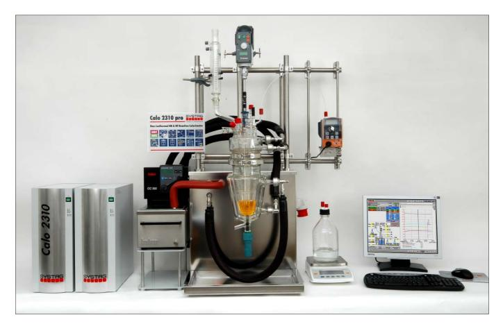
Combined **Heat Flow** and **Heat Balance Calorimeter** with automated "Zero Watt" Baseline for non-isothermal mode.
